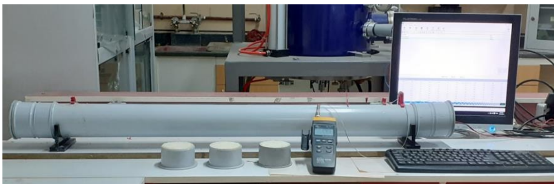
Figure 9. Impedance tube
